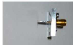
Common coax-waveguide transition (probe-feed)
