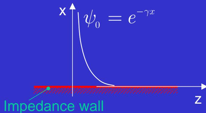
Surface wave of the open waveguide
