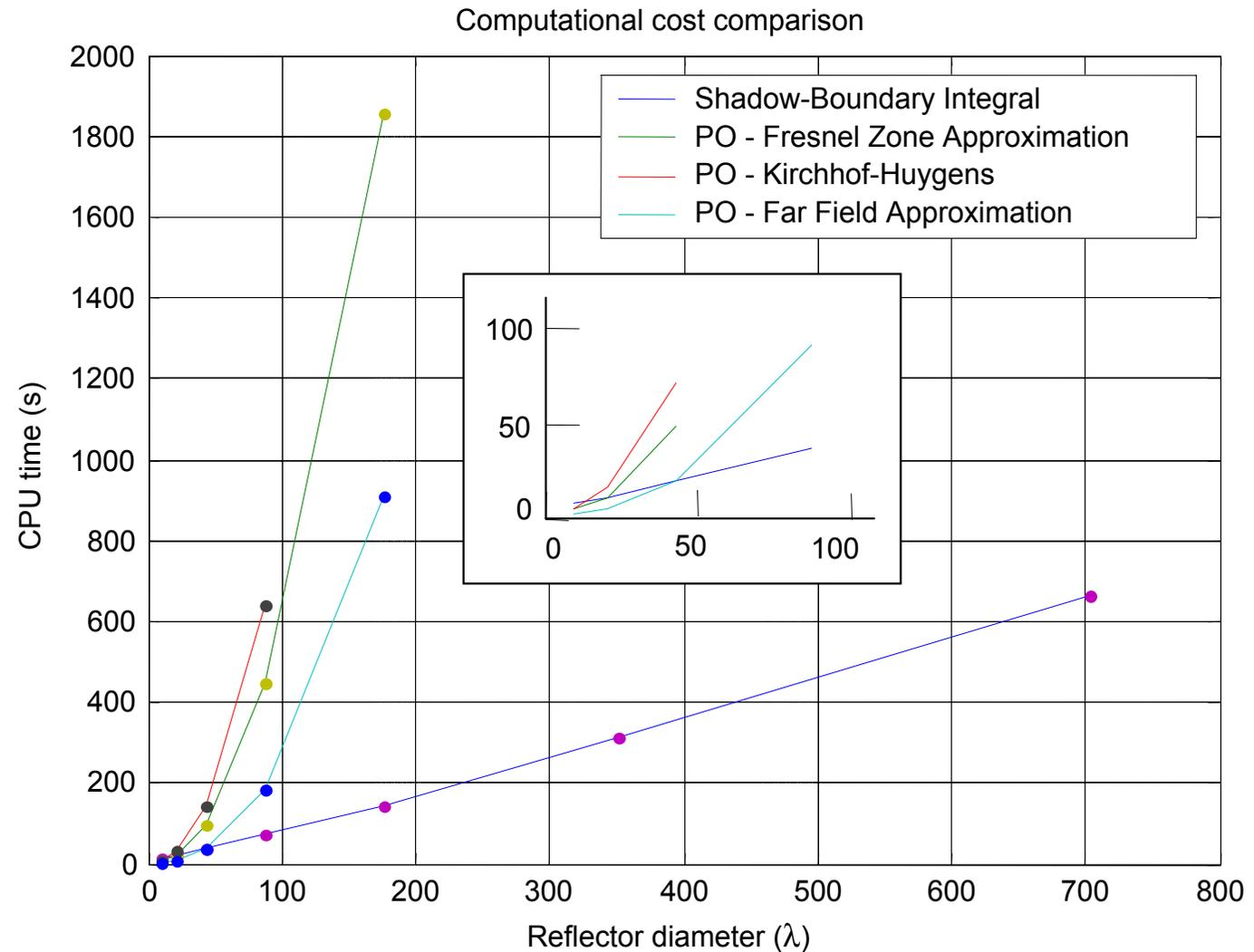
The dependence of CPU time on diameter of the antenna is linear
