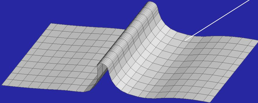
The trade off between good approximation and computational efficiency is solved by a non-uniform meshing
