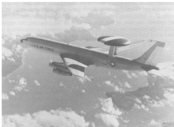
Figure 3.3-a: Slotted waveguide array in AWACS. Mechanically rotated in azimuth and phase steered in elevation.
