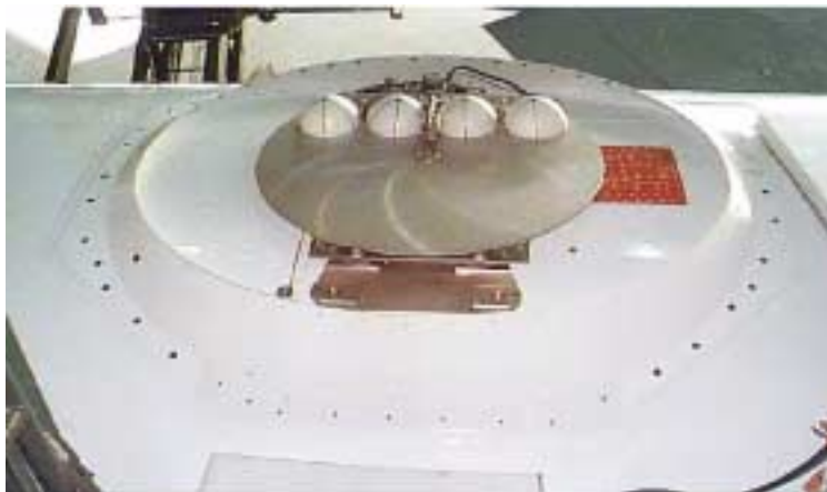
Figure 2.3-E : GBS/MILSTAR antenna consisting of a mechanically steered assembly of 4 lens hemispheres on a ground-plane.
