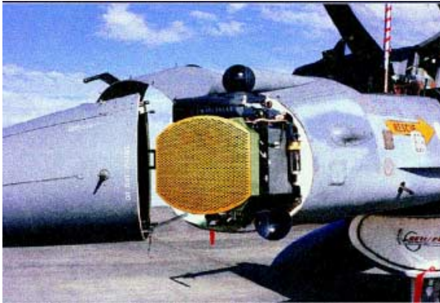
Figure 3.2-h: AN/APG-80 in F-16 Block 60, [VI].
