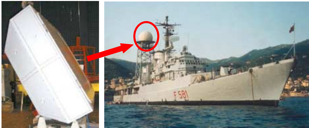
Figure 2.7-a: EMPAR System on the left (phase 2) and mounted inside a radome on the Italian ship Carabiniere. Alenia Marconi Systems, Italy.
