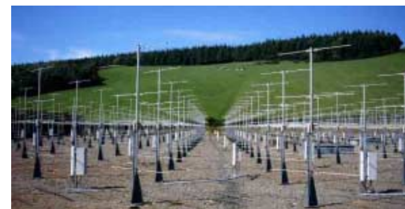
Figure 3-I : NERC MST radar facilities: a) 1290 MHz mobile boundary-layer wind profiler, b) 46.5 MHz Mesosphere-Stratosphere-Troposphere Radar.
