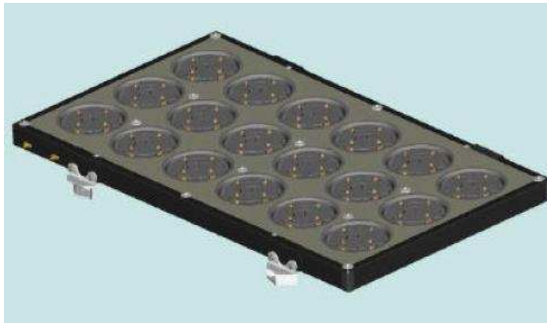
Figure 4.2-D SES dual frequency patch antenna for GPS occultation measurements [24].
