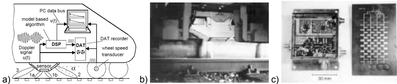
Figure 5-C : a) measurement setup, b) sensor on locomotive and c) radar front-end.
