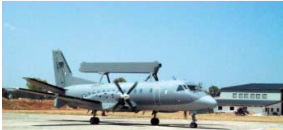
Figure 3.3-b: The ERIEYE with its pod with slotted waveguide on the back. Phased steered in azimuth.
