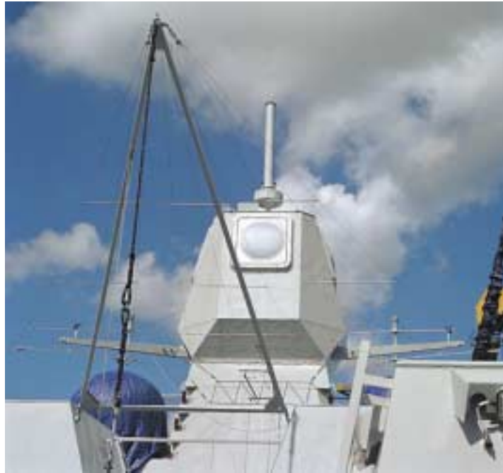
Figure 2.3-b: APAR mounted on ship. The polygonal tower contains all four array faces.
