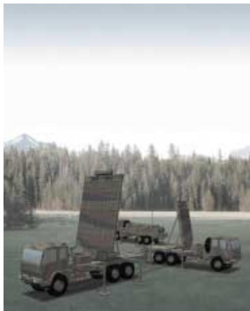
Figure 4.3-m: MEADS UHF Surveillance Radar and X-band Multifunction Fire Control Radar.
