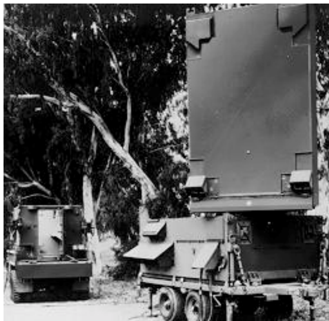
Figure 4.3-d : AN/TPQ-37 firefinder is a long-range weapon-locating radar.
