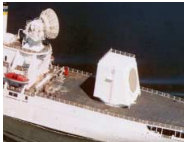
Figure 2.8-a: X-band dish antenna and the S-band phased array antenna system mounted on the USNS Observation Island.
