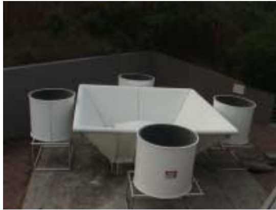
Figure 3-J : Integrated wind profiler and radio acoustic sounding system [81].
