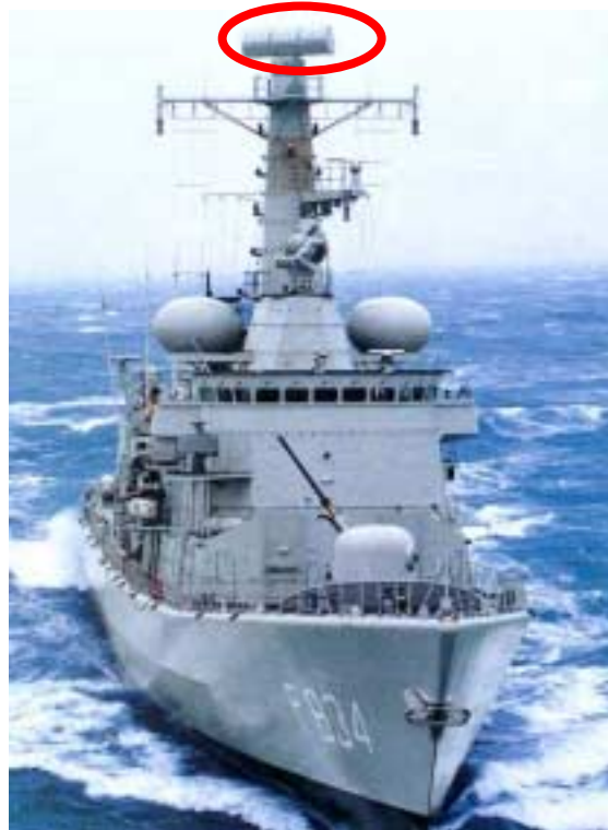
Figure 2.5-a: SMART-S mounted in the mast of the RNLN Frigate Karel Doorman.
