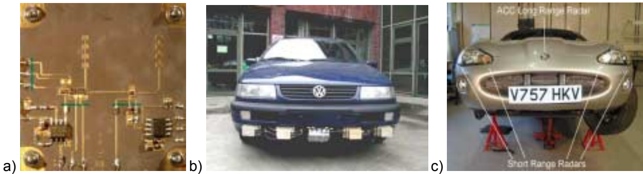
Figure 1-Q : a) photo of the 77 GHz RF module of the near distance RadarNet sensor [41], b) test vehicle with four 77 GHz RadarNet sensors [42], and c) example of radar network vehicle installation for the urban collision avoidance application [41]
