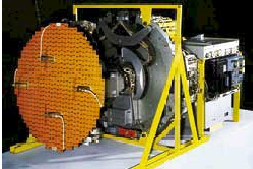
Figure 3.2-a: ZHUK-ME radar used in Mig 29 and Su 27, using a flat plate antenna, [I] (including four antennas for IFF).
