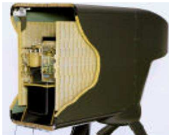
Figure 4.8-C Ericsson ERIEYE airborne early warning radar dorsal unit [14].
