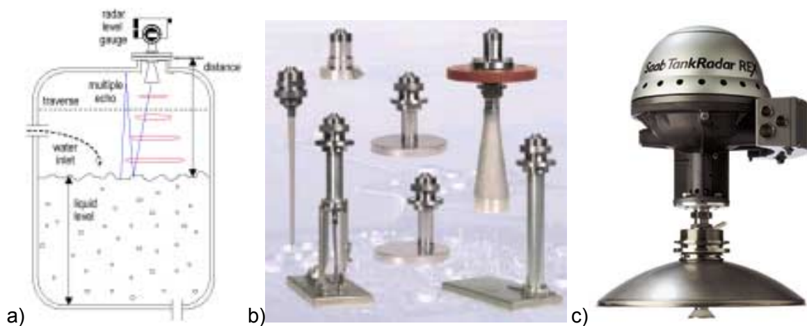
Figure 5-A : a) Radar tank level measurement [92], b) horn, dielectric rod, and planar antennas [93], c) radar level gauge [94].
