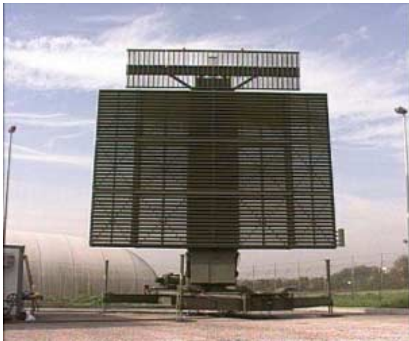
Figure 4.3-a : Air Defence and Battlefield System; Long Range Radar, RAT 31DL.
