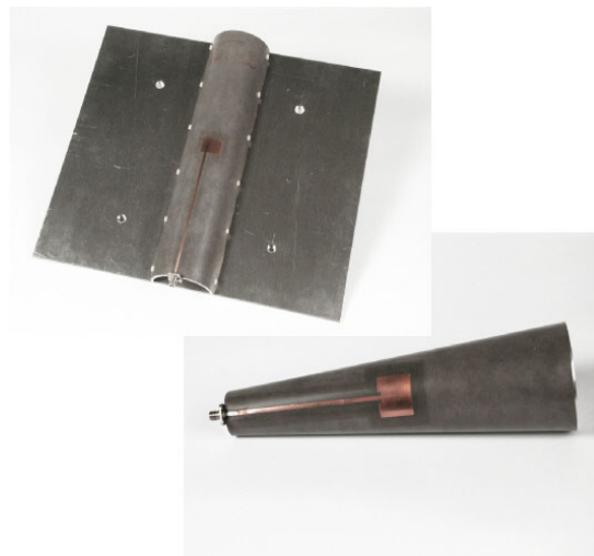
Figure 3.1-B. Cylindrical sector patch antenna and conical patch antenna built at DLR.
