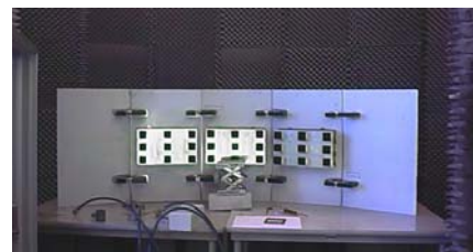
Figure 3.3-G. Variable faceted array of C-band open-ended square waveguides.
