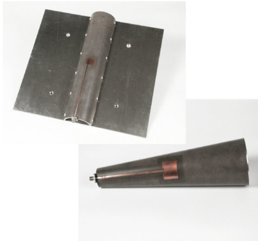
Figure 3.3-I. Cylindrical sector antenna and quasi-cylindrical antenna built at DLR.
