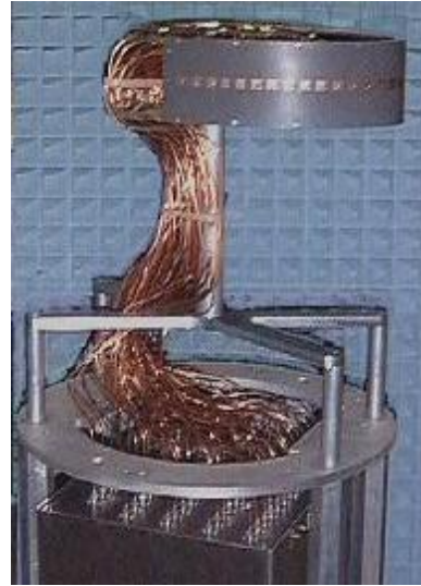
Figure 1.4-G. A demonstrator built at FGAN-FER, Germany. The picture shows a sector elliptical array and the upper part of the receiver [14].
