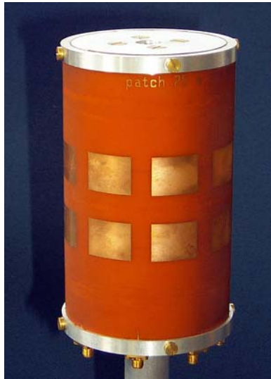
Figure 1.4-F. The experimental microstrip antenna built at the university of Karlsruhe, Germany [13].
