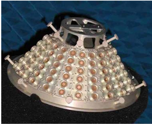
Figure 3.3-A. A conical satellite antenna built at Alcatel, France
