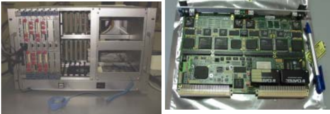
Figure 11. Software Defined Radio platform with 4292 Pentek boards
