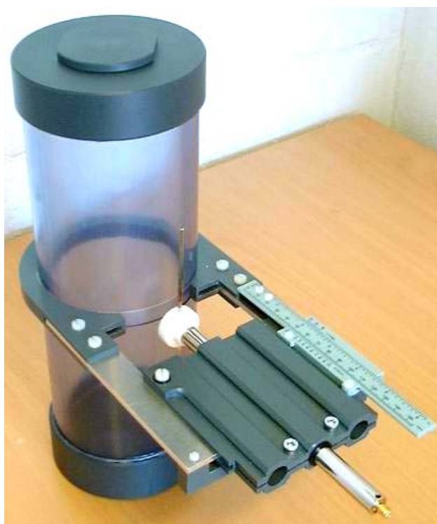
Fig. 13. The single dipole close to lossy cylinder efficiency measurement setup.
