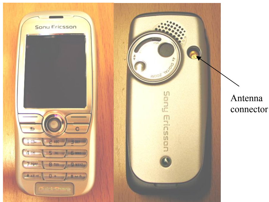
Fig. 4. Special phone for total radiated power measurements. Front and backside, respectively.
