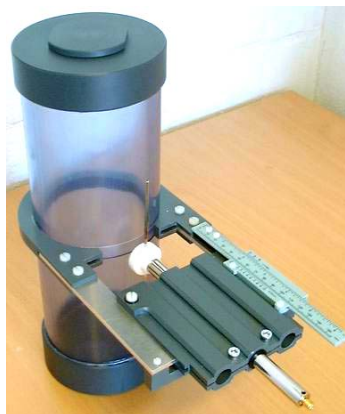
Fig. 4.1.1. Test setup for efficiency measurement – Single dipole close to lossy cylinder.
