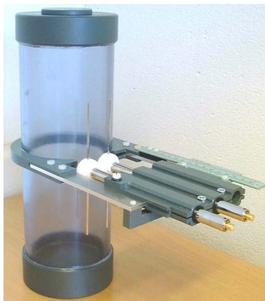
Fig. 2. Passive device test setup – Two dipoles for diversity measurements.
