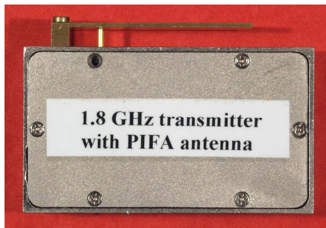
Fig. 5. Active device radiating at 1.785 GHz used for total radiated power measurements.
