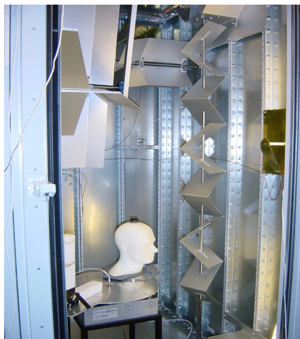
Fig. 5.9.1. Scattered field chamber used by SES.
