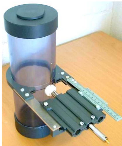
Fig. 1. Passive device test setup – Single dipole for efficiency measurements.
