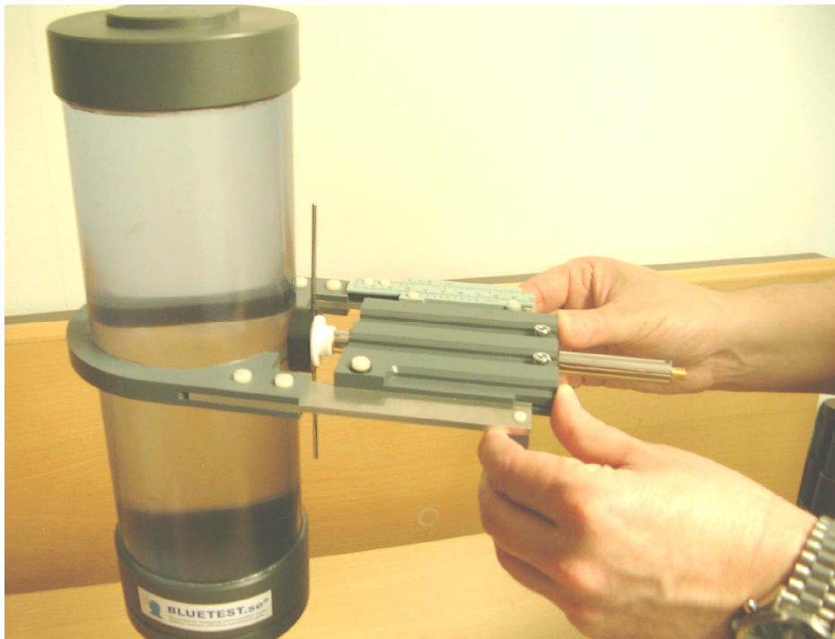
Fig. 9. Dipole spacer pressed against the cylinder. This corresponds to a distance of 10 mm between the dipole and the cylinder.
