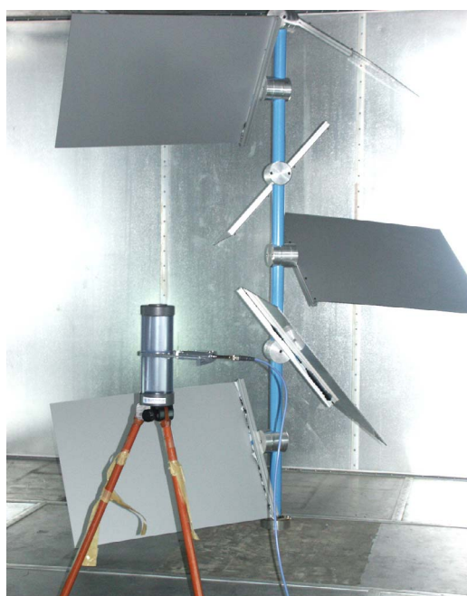
Fig. 5.8.1. Reverberation chamber used by IETR.
