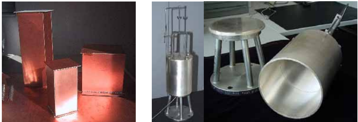
Figure 24: Wheeler-cap measurement setups.
