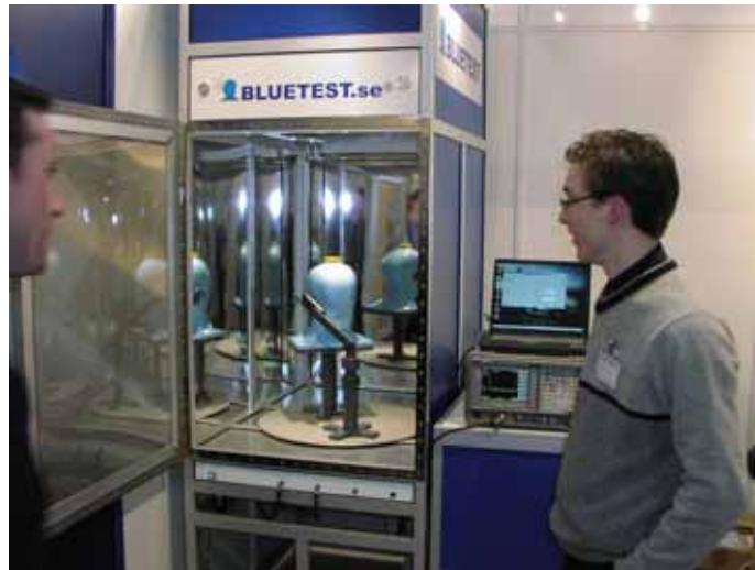
Figure 18. The Bluetest reverberation chamber shown with open door with a setup for measuring radiated power of mobile phone close to head phantom. The chamber size shown can be used for measurements down to 850 MHz.
