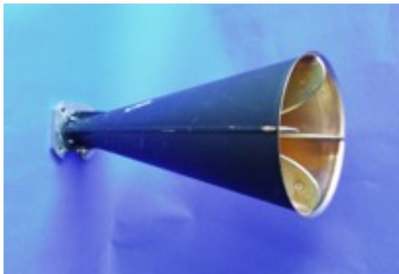
Figure 16: Quad-ridged horn (reference antenna)
