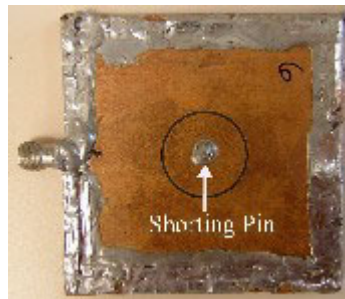
Figure 34: Cavity backed annular slot with a shorting pin
