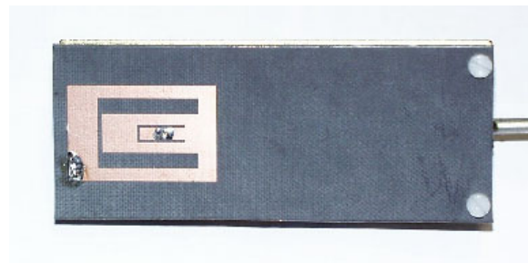
Figure 66: Photo of the handset PIFA prototype.
