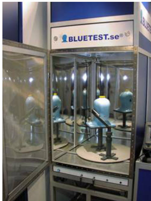
Figure 12: Measurement of user interaction in reverberation chamber
