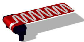
Figure 22: Meander line antenna.
