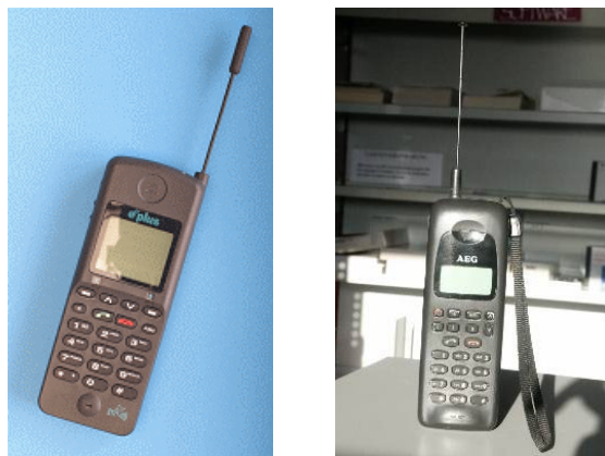
Figure 19: Terminals with \lambda/4 monopole antenna.
