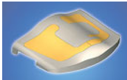
Figure 29: Typical structure of a 3D-MID antenna.
