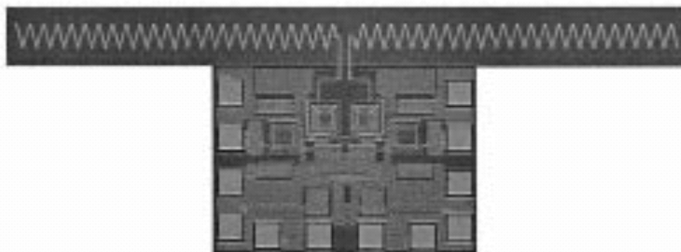
Figure 3.3.13: Die photograph of a 0.18 \mu m clock receiver with a 2 mm zigzag dipole antenna.
