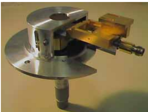
Figure 4.3-19: a GBA with its measurement setup at 60 GHz
