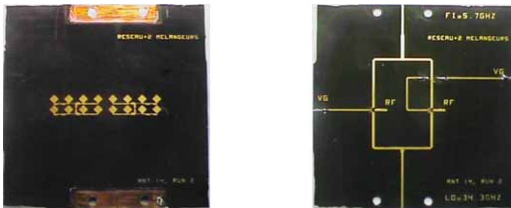
Figure 4.3-1: Active antenna with mixers
