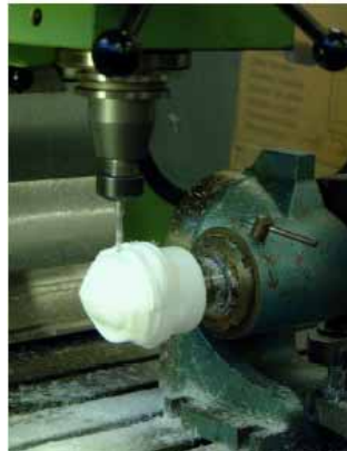
Figure 4.1-19: Fabrication of a Teflon lens (Fig. 5) on a milling machine [7]
