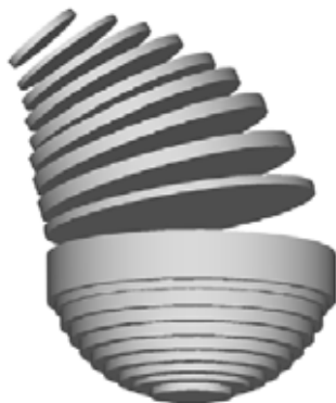
Figure 4.1-23: A sliced spherical Lüneburg lens operating around 30 GHz [20]
