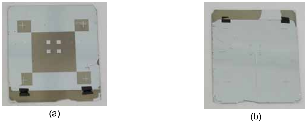
Figure 4.3-4: Front (a) and rear (b) view of an aperture-coupled microstrip patch antenna array printed on 150μm-thick fused quartz substrates
