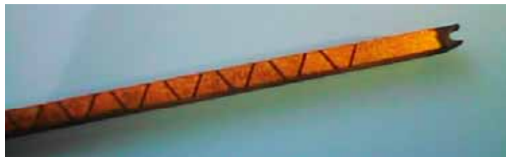
Figure 4.3-15: Transversal slot waveguide antenna
