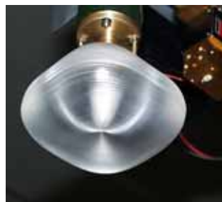
Figure 4.1-21: Quasi BoR shaped lens antenna at 62.5 GHz [18]
