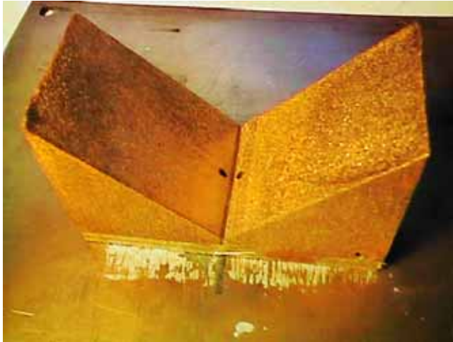
Figure 4.3-13: 3D V dipole antenna
