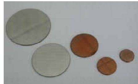
Figure 4.3-18: Examples of FP cavities with inductive patterns
