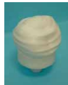
Figure 4.1-22: Optimized 3D shaped lens at 58 GHz [19]
