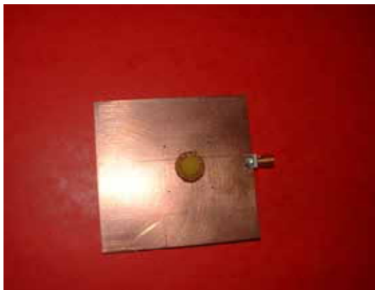
Figure 4.3-9: Technology of the multifrequency dielectric resonator antenna
