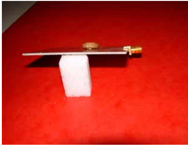
Figure 4.3-8: Geometry of a multifrequency dielectric resonator antenna
