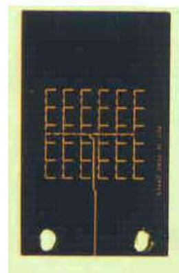
Figure 5b : Feeding lines network Amplitude taper : (0.3; 0.7, 1, 1, 0.7, 0.3) in the two planes.
