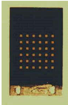
Figure 5a : Radiating array spacing between patches : 0,72 \lambda_0
