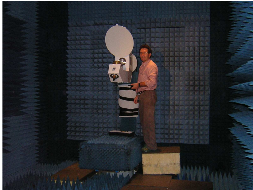
Figure 3.5 VAST12 in LEHA-UPM Spherical near-field system.
